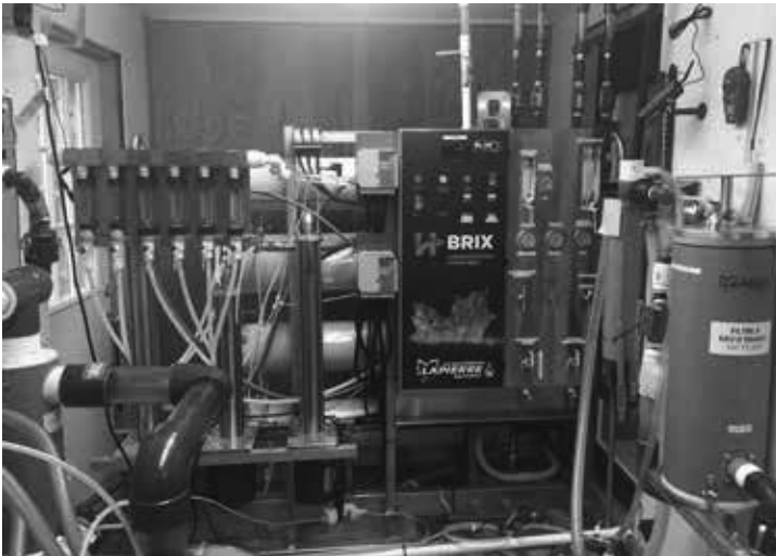
Figure 1. Lapiere Equipment HyperBrix Reverse Osmosis machine in operation at the Sumner Hill Williams research/demonstration sugarculture at UVM PMRC in 2018. Note the flow-meters and inline refractometer on lines in the upper right of photo. Photo Credit: Timothy Perkins, UVM PMRC.
